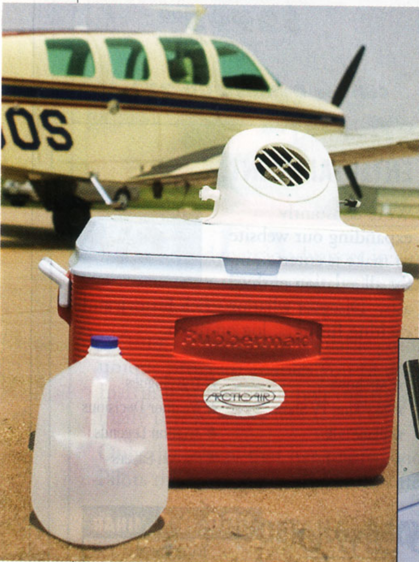
A gallon of water, bags of ice, a fan, pump, and plumbing turn an ice chest into an ArcticAir air conditioner.
