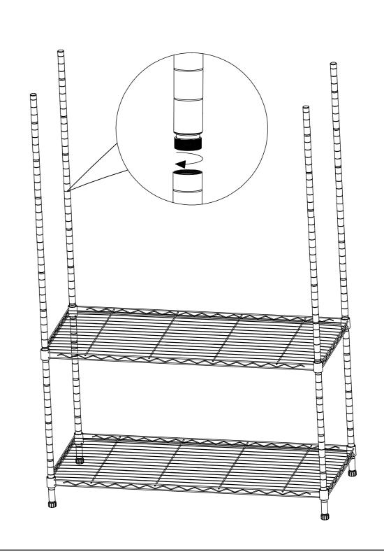
Once all shelves have been installed firmly push down or tap gently with a rubber mallet to ensure all shelves are securely on the Plastic Clips. Place polypropylene mats on to the shelves.
