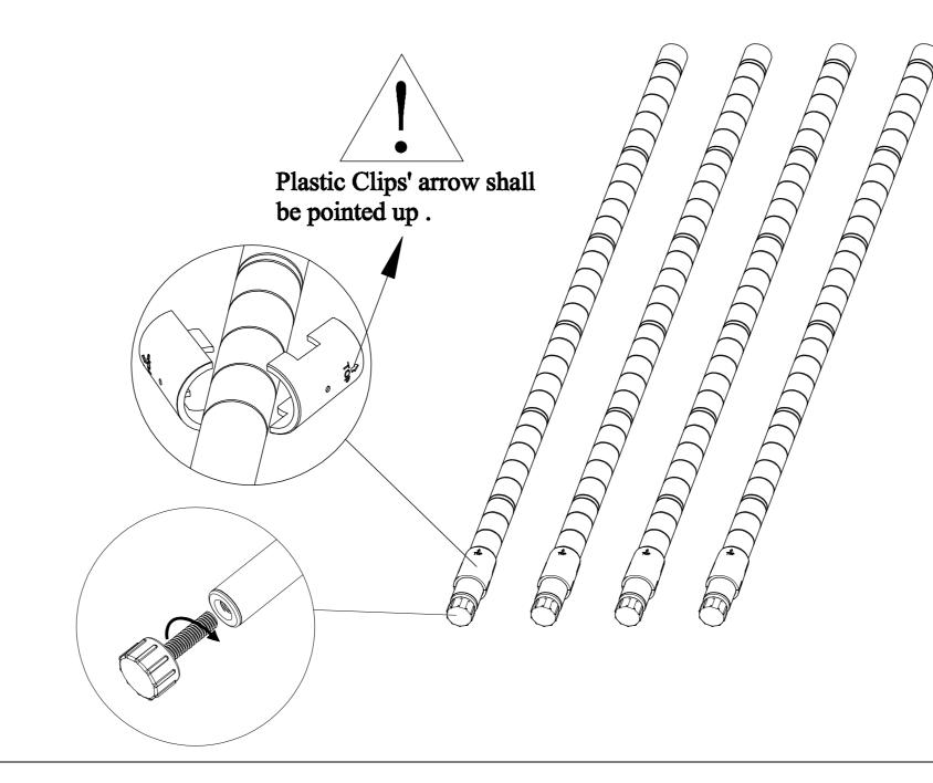
NOTE: The exact location of the shelves is the customer's preference. We recommend you consider what will be on the shelves and the spacing you will need before assembling the unit completely. Snap 8 Plastic Clips (E) on the pole grooves of the 4 Lower Poles. Then slide down a Wire Shelf (A) onto the plastic clips.
