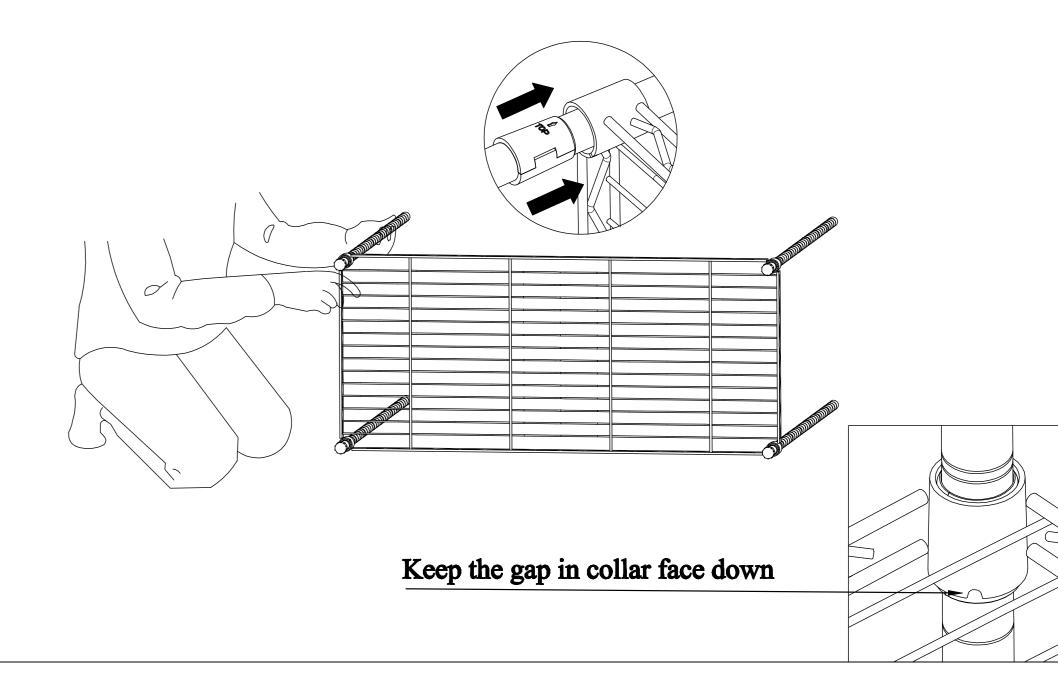
Screw Upper Poles (C) into the Lower Poles as shown.
