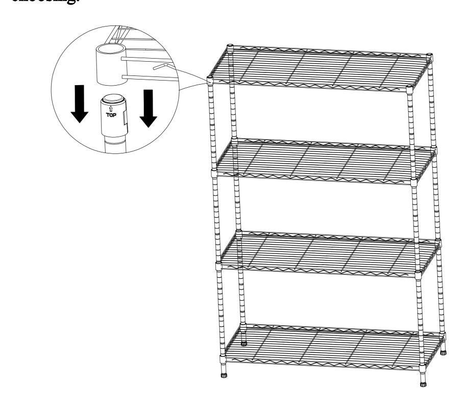
Please make sure the Wire Shelf (A) is positioned correctly (as shown). Hold the shelf on its side and slide the four Lower Poles (B) through the bottom of the shelf through the holes in the corner until they fit snugly. Once the four Lower Poles are securely through the holes, set the shelf upright.
