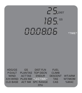
After **LEG TIME** is calculated, the count down timer can be activated starting at the calculated time by pressing
