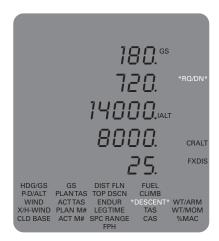
**Note:** This **ATC** crossing restriction will require a descent rate of 720 feet per minute. A positive value for **RQ/DN** indicates a descent. A negative value indicates a climb to the crossing altitude.
