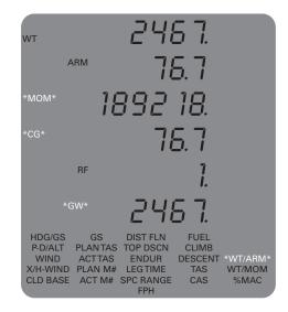
After keying in the airplane's empty weight and arm, the next step is to calculate the weight and balance for the aircraft at takeoff. For this example, we'll assume the following load:
