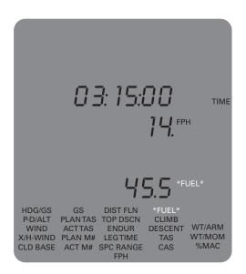
**Note**: The Fuel Required function computes fuel consumption only; it does not take required fuel reserves into account.
