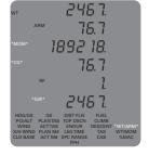
After keying in the airplane's empty weight and arm, the next step is to calculate the weight and balance for the aircraft at takeoff. For this example, we'll assume the following load:
