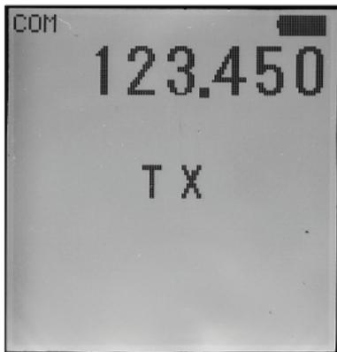
Release the PTT to end the transmission and the PJ2 COM will once again receive the selected COMM frequency. If a headset is being used, the PJ2 COM's internal microphone will be deactivated and the microphone on the headset may be activated by either pressing the PJ2 COM's PTT or pressing an inline remote PTT.
