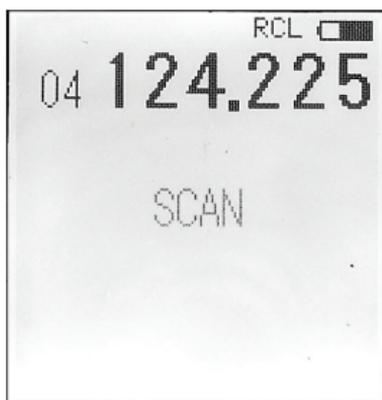
When a broadcasting signal is found, the word SCAN will flash and the PJ2 COM will stop temporarily on that frequency. If the broadcasting signal is cut off for more than two seconds, the Scan will resume until another signal is found.
