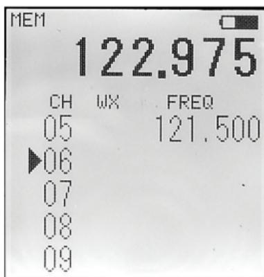
The first available memory channel will be displayed with an arrow on the screen. In this example, memory channel 06 is the first available location. To store the frequency, press the Memory Key a second time. The screen will now display the following for one second to verify 122.700 has been stored in memory channel 01.
