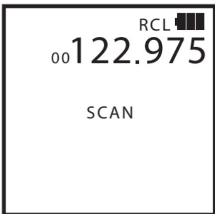
When a broadcasting signal is found, the word SCAN will flash and the SP-400 will stop temporarily on that frequency. If the broadcasting signal is cut off for more than two seconds, the Scan will resume until another signal is found.
