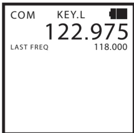
Key Lock is deactivated by holding the Clear Key and pressing the Down Key a second time. Key Lock only locks out the SP-400's keypad. The PTT and Light functions are not affected.
