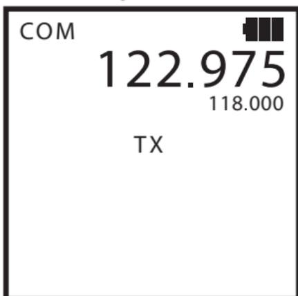
Release the PTT to end the transmission and the SP-400 will once again receive the selected COMM frequency. If the optional Headset Adapter is being used, the SP-400's internal microphone will be deactivated and the microphone on the headset may be activated by either pressing the SP-400's PTT or pressing an inline, remote PTT.
