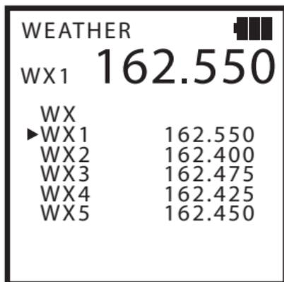
At this point you may select any stored weather channel by pressing the Up or Down Key to scroll through the stored frequencies. Weather channels may also be accessed directly by using the Numeric Keypad. For example, to receive weather channel 08 you may either:
