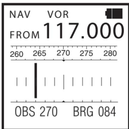
The OBS setting will remain set to the initial bearing or radial until otherwise changed. The CDI needle will continuously update to show the deviation from the selected radial as the aircraft moves.
