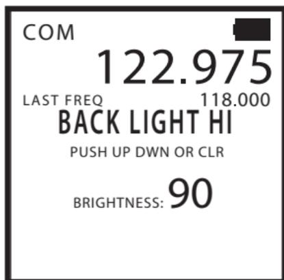
Once in high back light mode, the back light can be further adjusted from level 10 to level 99 by pressing the up or down keys.
