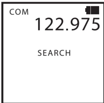
The frequencies will either scroll up or down in 8.33 KHz steps depending upon whether the Up or Down Key was used to initiate the Search.
