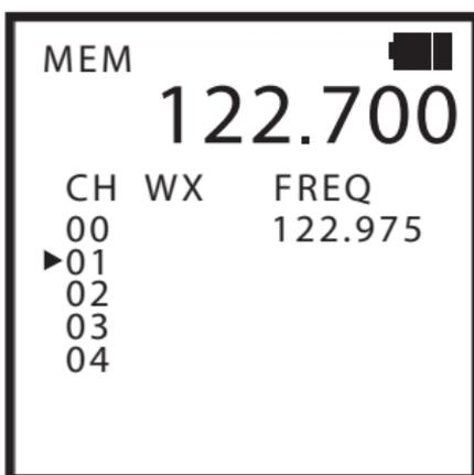
The first available memory channel will be displayed with an arrow on the screen. In this example, memory channel 01 is the first available location. To store the frequency, press the Memory Key a second time. The screen will now display the following for one second to verify 122.700 has been stored in memory channel 01.
