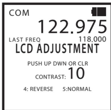
The contrast can be adjusted by pressing the up or down keys. Press the clear key to save the setting.
