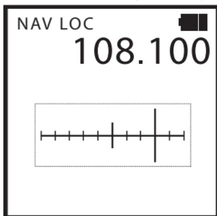
The Course Deviation Indicator (CDI) is displayed on the screen. When receiving a Localizer signal, each division on the CDI represents a one degree deviation. Therefore, the CDI on the SP-400 has the ability to display up to a 5 degree deviation to the right or left in Localizer mode. The above example shows a 3 degree deviation to the left (fly right towards the needle to be on course). OBS and BRG are disabled in LOC mode.
